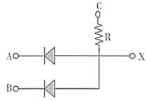
Figure 3.9: Diode AND Gate
