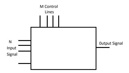
Figure 4.15: Multiplexer Pin Diagram
