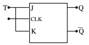
Figure 5.6: T Flip Flop using J K Flip Flop
