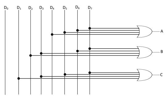
Figure 4.12: Octal to BCD Encoder Circuit
