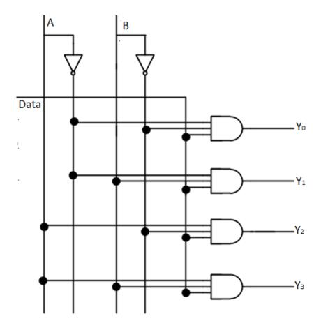
Figure 4.18: DeMultiplexerCircuit Diagram
