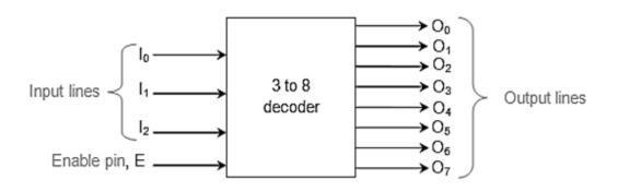
Figure 4.13: Decoder Block Diagram
