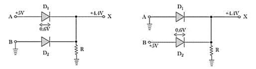
Figure 3.5: Diode OR Gate with any one input is +5v
