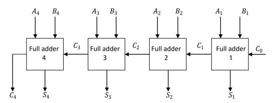
Figure 4.5: Binary parallel Adder
