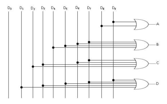
Figure 4.11: Decimal to BCD Encoder Circuit
