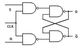
Figure 5.2: Clocked RS Flip Flop
