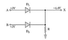
Figure 3.6: Diode OR Gate with both inputs are +5v
