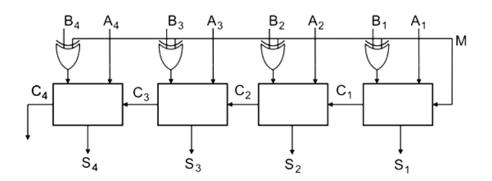
Figure 4.9: Four bit Full adder and Subtractor
