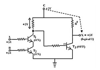
Figure 3.12: Transistor AND Gate
