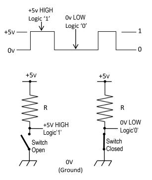
Figure 3.2: Digital Logic Gate Voltage Level
