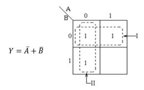
Pairs of 1's are grouped as shown above, and the simplified answer is obtained by using the following steps: Two groups can be formed that the largest rectangular bands that can bemadeconsistoftwo1s.
