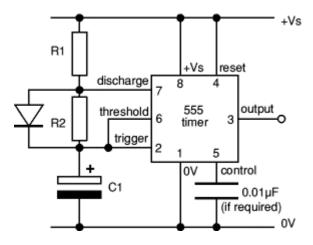
Figure 5.14: 555 Astablecircuit with diode across R2 Tm can be less than Ts so the duty cycle can be less than 50%
