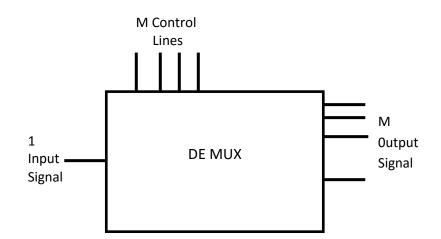
Figure 4.17: DeMultiplexer Pin Diagram
