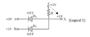
Figure 3.10: Diode AND Gate with both input +5v
