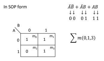
Result of  $\overline{AB} + \overline{AB} + AB$  is  $\overline{A} + B$
