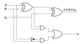
Figure 4.4: Full Subtractor Circuit
