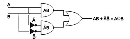
Figure 3.27 Logical Circuit diagram of XNOR Gate
