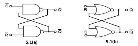
Figure 5.1: Latch RS Flip Flop Using NAND and NOR Gates
