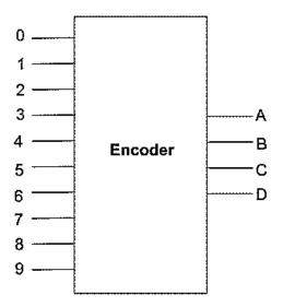
Figure 4.10: Encoder Block Diagram
