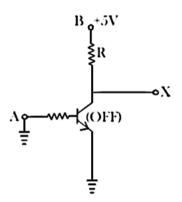
Figure 3.15: Transistor Circuit NOT Gate and with input 0v
