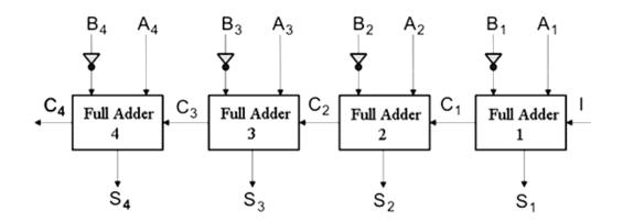
Figure 4.6: Binary Subtractor Circuit
