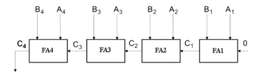
Figure 4.7: Four bit Full adder
