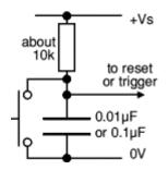
Figure 5.19 : For Automatic Trigger
