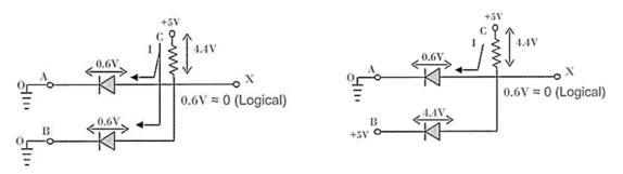
Figure 3.11: Diode AND Gate with any one input +5v
