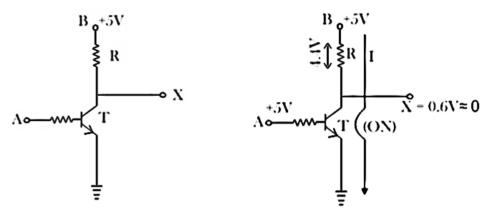
Figure 3.14: Transistor Circuit NOT Gate and with input +5v
