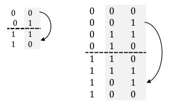
Process of obtaining 4 bit Gray code by reflecting 3 bit Gray code:
