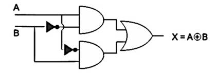
Figure 3.25 Logical Circuit diagram of XOR Gate
