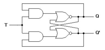
Figure 5.5: T Flip Flop
