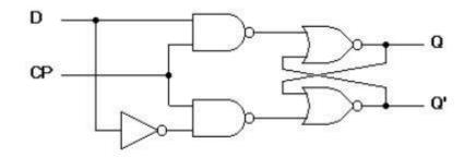
Figure 5.3: D Flip Flop
