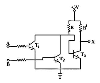
Figure 3.7: Transistor OR Gate
