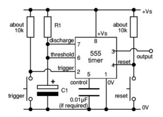
Figure 5.17: 555 monostablecircuit with manual trigger
