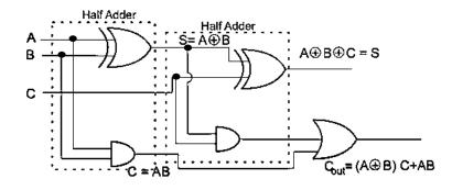
Figure 4.2: Full Adder Circuit
