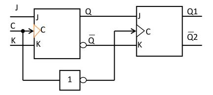
Figure 5.8: Master Slave JK Flip Flop (Block diagram)
