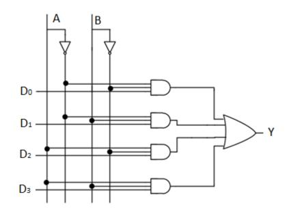
Figure 4.16: Multiplexer Circuit Diagram
