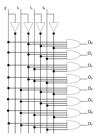
Figure 4.14: Binary Decoder Circuit using Basic Gates
