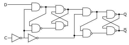
Figure 8(a): Master Slave Flip Flop
