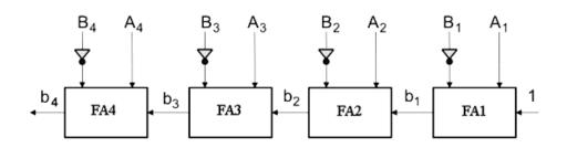
Figure 4.8: Four bit Full Subtractor
