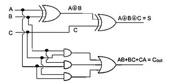
Figure 4.2a: Full Adder Circuit
