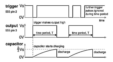
Figure 5.18: 555 monostable Operation
