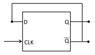
Figure 5.7: D-type Flip Flop connected as toggle stage
